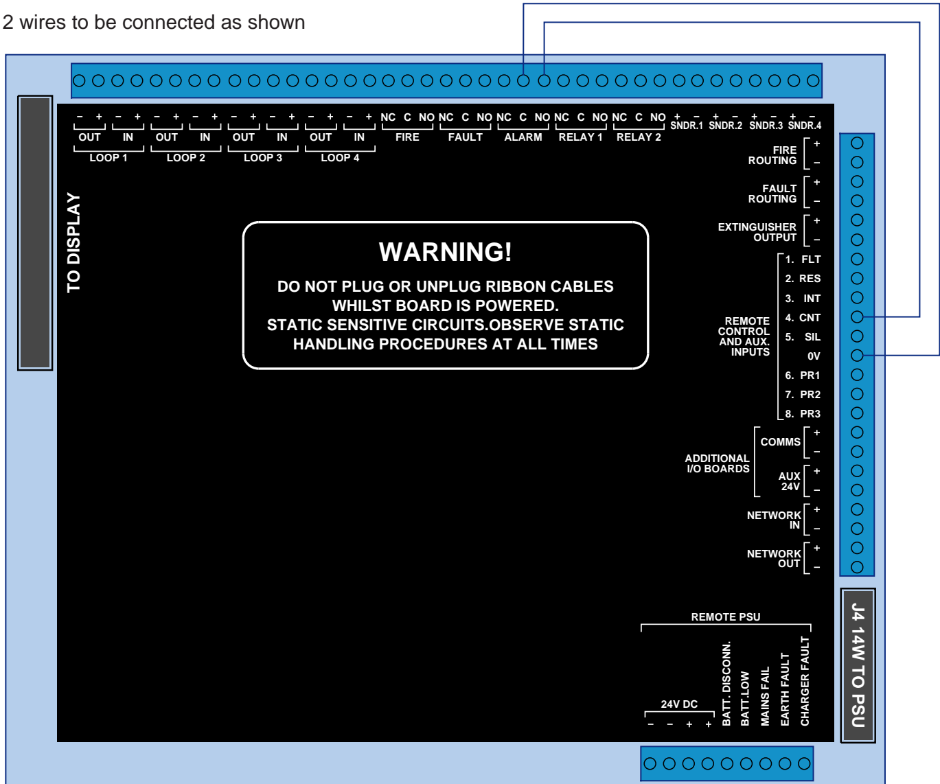
Fig 1 - Panel hardware connections
